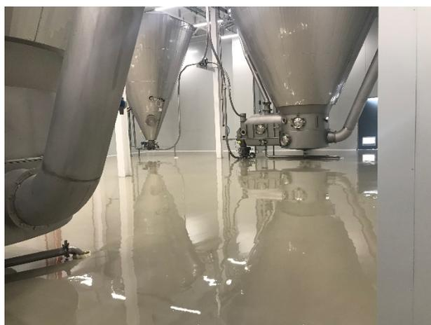
*Image: "Industrial dryers used to spray dry blood"*
